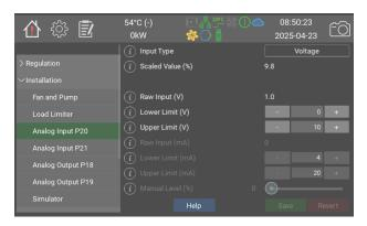
The analog inputs can be used to control set temperature, power limit, DPC power etc.
