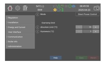
The boiler's overtemperature protection should be set to trip a few degrees below the external overheating protection. When the overtemperature protection triggers, the contactors are shut off and a yellow warning shows. Normal regulation resumes when the boiler temperature has fallen below "Hysteresis (°C)" hysteresis.
