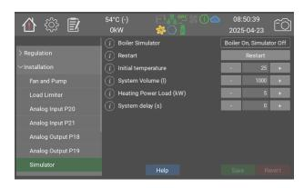
The simulator can be used fo demoing and is useful for testing input and output signals before deploying the boiler.
