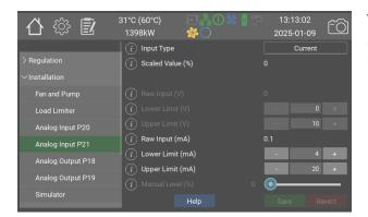
The analog inputs can be used to control set temperature, power limit, DPC power etc.
