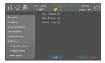
This page shows the actual current/ phase at the fuses the load limiter protects. For correct display, it is required that all settings regarding the load monitor are correctly performed and adjusted.
