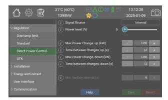
DPC enables direct power control from a superior control system. In this mode, the internal temperature control is switched off. Overheating protection, maximum installed power and any external power limitation apply.
