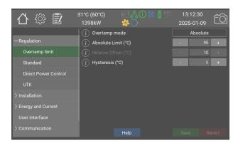
The boiler's overtemperature protection should be set to trip a few degrees below the external overheating protection. When the overtemperature protectione is activated, the contactors are shut off and a yellow warning shows. Normal regulation resumes when the boiler temperature has fallen below "Hysteresis (°C)" hysteresis. Current limit value can be set to an absolute value or a relative value that follows Actual Setpoint Used, up and down.
