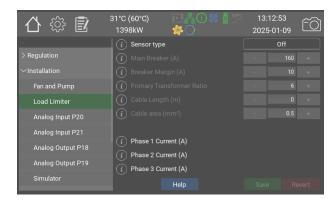
The load limiter protects the main fuses. The boiler continously measures the current at the junction box and and adusts the output power so that the total current stays below a defined threshold.
