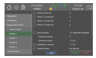
Each busbar has a current measurement board. This board measures the current on the three phases and any imbalance between them.
