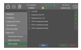
Status of other inputs and outputs on the main board, and on the expansion board
