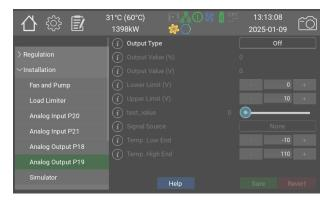
The analog outputs can be used to read an internal process value. The output
