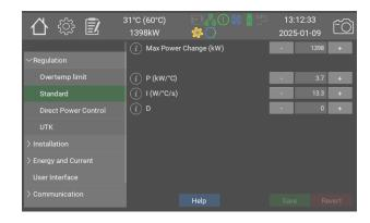
In standard mode, the goal is to keep the boiler temperature as close to the setpoint as possible. The boiler regulates best if it is allopwed to jump freely between availabe steps, but it is possible to limit the jump size if the installation requires it.
